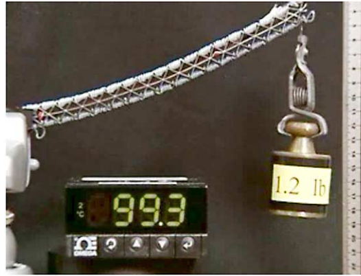
Fig. 8. Prototype (200 mm length) beam, fixed in vise at left, lifting 1.2 lb (540 g) a distance of 92 mm. The thermocouple shows temperature (°C) of the active (top) SMA face.
